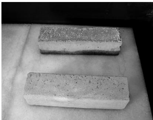
Fig. 5 Test specimen for water up-take measurement were placed on a water saturated PU-foam. The specimen in the upper half is untreated whereas the specimen lower half is treated with Additive 3 powder.
